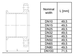
Threaded socket according to DIN 11851
