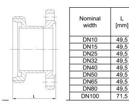
Conical socket with groove nut according to DIN 11851
