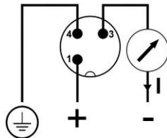
Assignment of the M12 device plug
