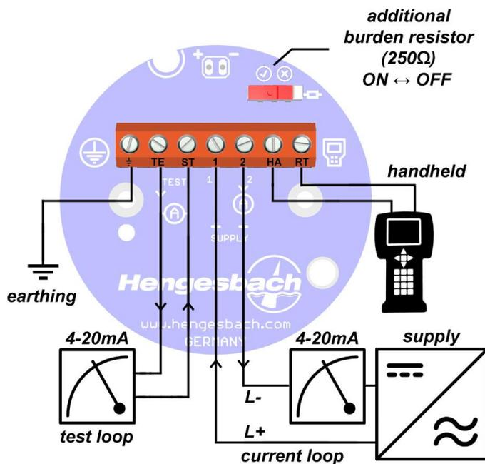
Connection diagram for a device in 200H/201H version
